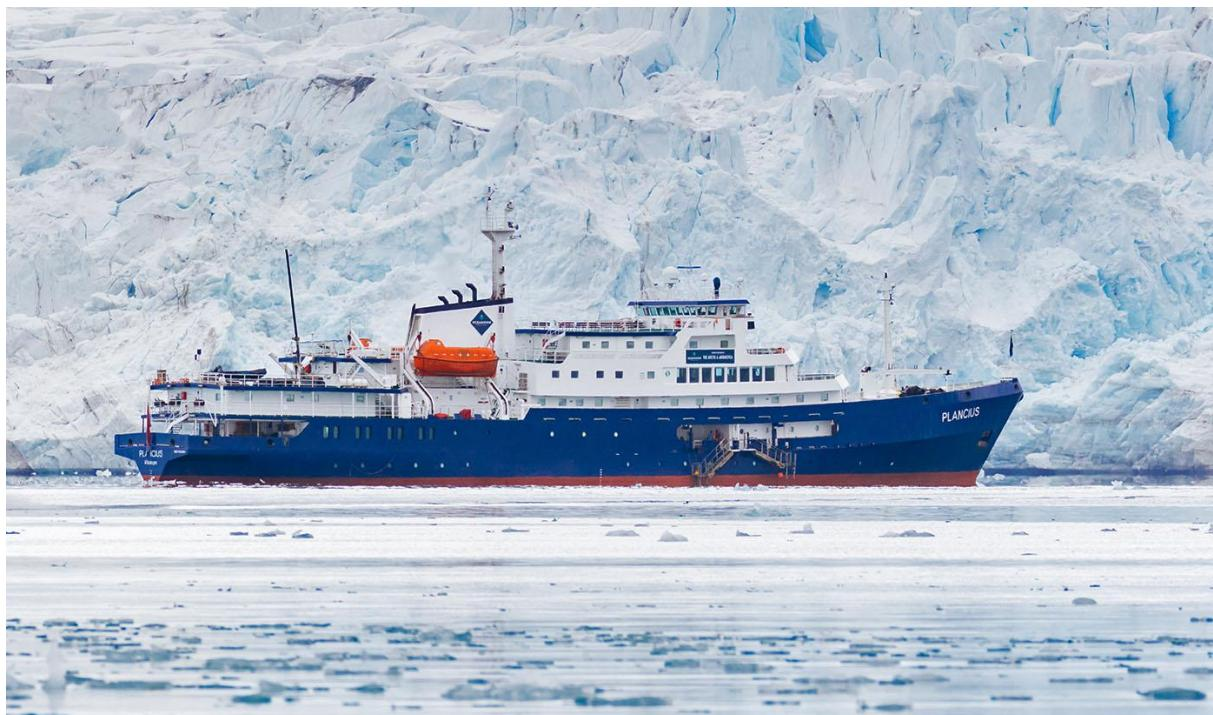
M/v *Plancius* was built in 1976 as an oceanographic research vessel for the Royal Dutch Navy and was named “Hr. Ms. *Tydemans*”. The vessel was completely rebuilt as a passenger vessel in 2009 and complies with the latest SOLAS-regulations (Safety Of Life At Sea). M/v *Plancius* is 89 m long, 14.5 m wide and has a maximum draft of 5 m, ice class 1D, 10,5 knots average cruising speed and has 3 Diesel- Electric engines.
